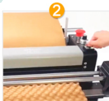
2 Start up the machine and adjust the speed
