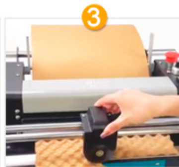
3 Tear by hand or with slide cutter to cut the paper bubble
