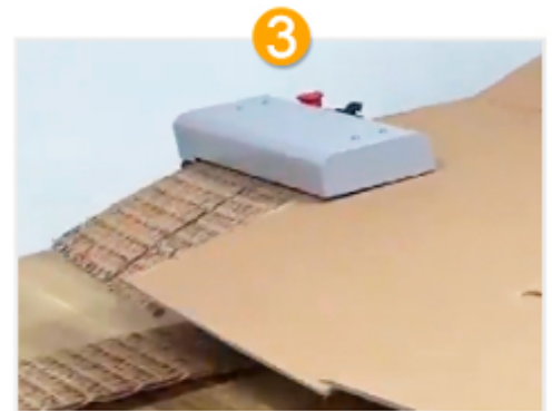
3 Place the cardboard into the paper inlet, and start cutting
